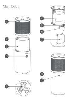
1. Metal cover 2 Ventilation hole 3. Water tank 4. Water marker 5. LED Light 6. Mist chip 7. Fan 8. ON/OFF. Time setting 9. Battery LED indicator 10.USB port 11. Air inlet 12. Power adapter 13. Type-C USB
